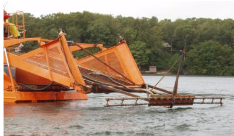
Manifolds before lowering to treatment depth.
